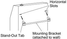
Figure 10 - Mounting Heater Onto Mounting Bracket
